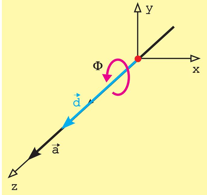
$$\bar{R}_z(\phi) = \begin{pmatrix} \cos\phi & -\sin\phi & 0 & 0 \\ \sin\phi & \cos\phi & 0 & 0 \\ 0 & 0 & 1 & 0 \\ 0 & 0 & 0 & 1 \end{pmatrix}$$
