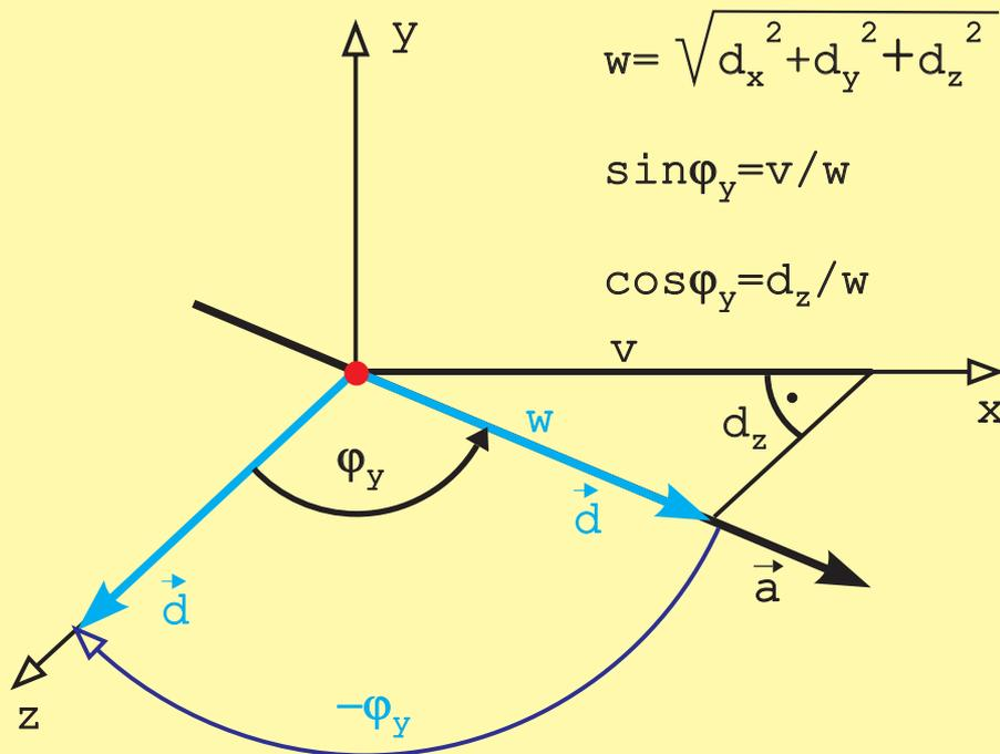
$$\overline{R}_Y(-\varphi_y) = \begin{pmatrix} d_z/w & 0 & -v/w & 0 \\ 0 & 1 & 0 & 0 \\ v/w & 0 & d_z/w & 0 \\ 0 & 0 & 0 & 1 \end{pmatrix}$$
